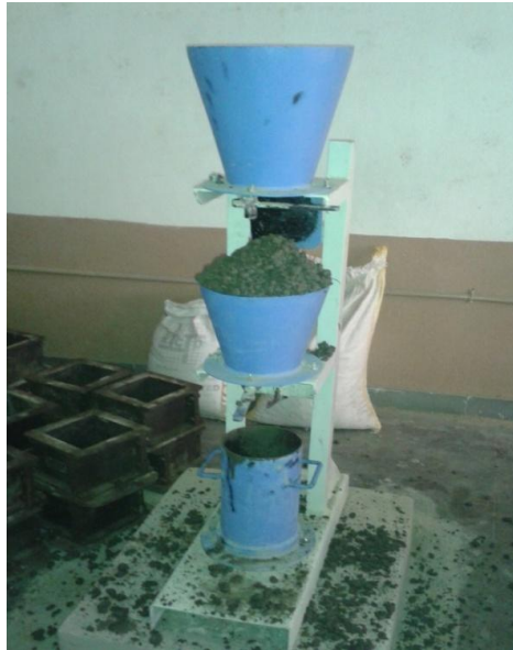
Fig- 10 : Workability test
