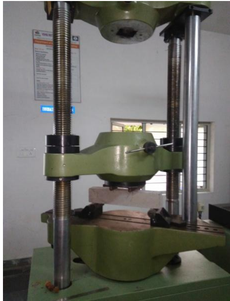
Fig-7: Flexural strength test
