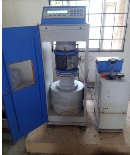
Fig-1: Compressive strength test
