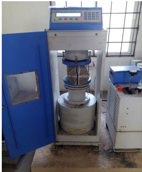
Fig-4 : split tensile strength test
